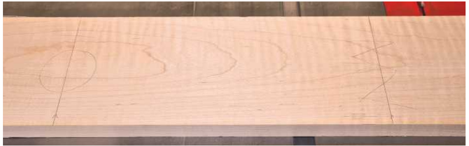
▲ Pic.3 For this project I decided to use a tiger maple board, which measured 1,524 × 125 × 20mm. I cut four pieces measuring 305mm long with 45° corners. So the grain pattern could be followed as you turn the box, I marked each of the four sides with directional arrows. Next, I cut a slot 3mm from the top of each piece, 7mm wide and 6mm deep, which would accommodate the walnut lid section. I wanted the lid to float in the slots for wood movement so no glue was used on the walnut
